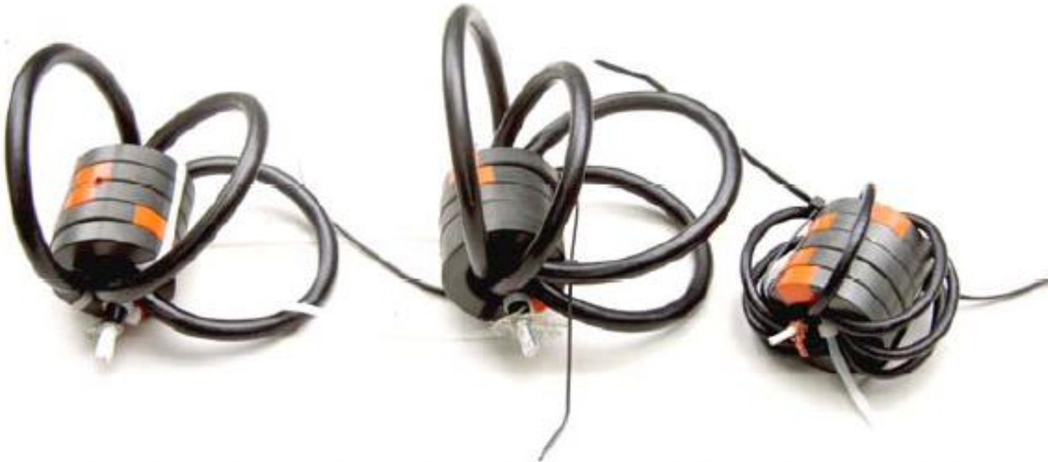
Fig 36 – Coaxial Chokes Wound to Minimize L and C
