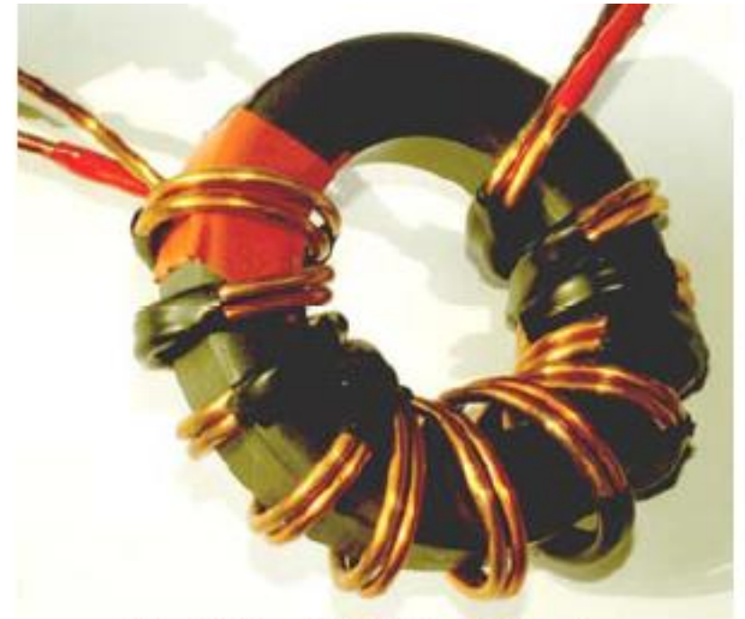
Fig 37 – A Bifilar Choke
