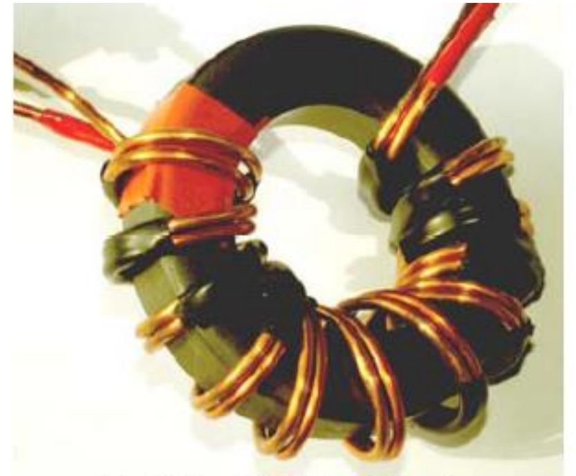
Fig 37 – A Bifilar Choke
